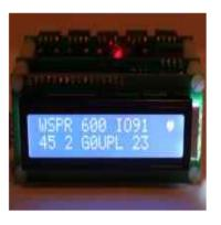
The Ultimate3S QRSS/WSPR Transmitter Kit is the new edition of the third version in the "Ultimate" QRSS/WSPR kit trilogy. It can produce QRSS, Hell, WSPR, Opera and PI4 slow-signal modes anywhere from 2200m to 2m and even 222MHz bands. Plug-in LPF filters are available for all 16 HF/MF/LF/VHF bands from 2200m to 222MHz.
